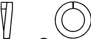
Key # ④ spring lock washer 10mm QTY. 4
